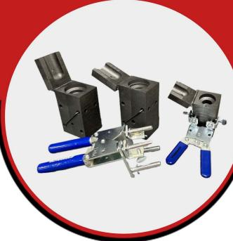
Mine Cable Services offers Exothermic Molds, Welding Charges, and Tool Kits in complete kits sized to your specific cable, or as individual replacement components.
